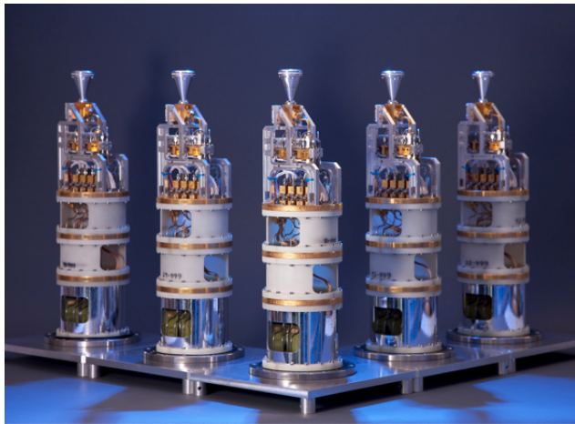
FIG. 1.— A collection of Band 3 receivers at NRC-HIA.
