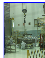
Fig. 1: WFC3 is moved from the clean room to the vacuum chamber. Credit: H. Bushouse
