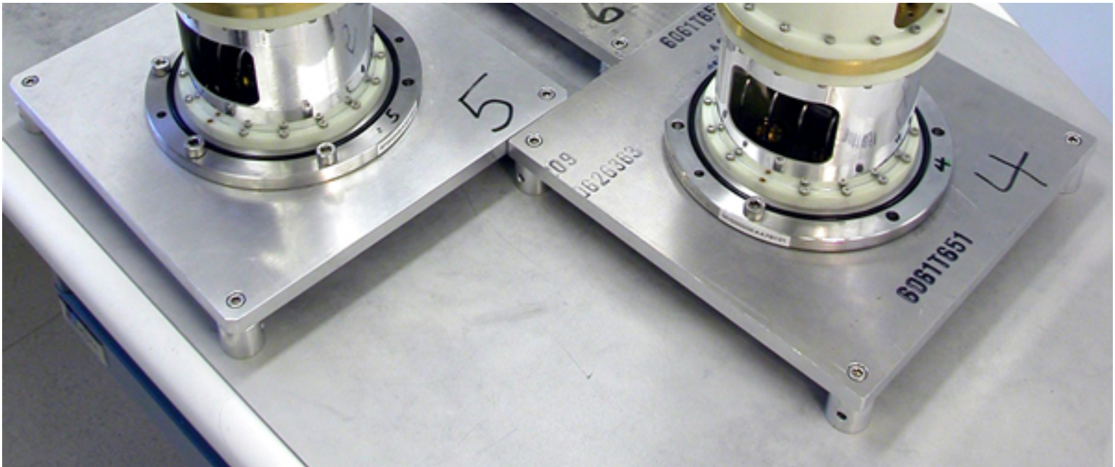
Figure 3: Four ALMA Band 3 receiver cartridges that are under construction at HIA.
