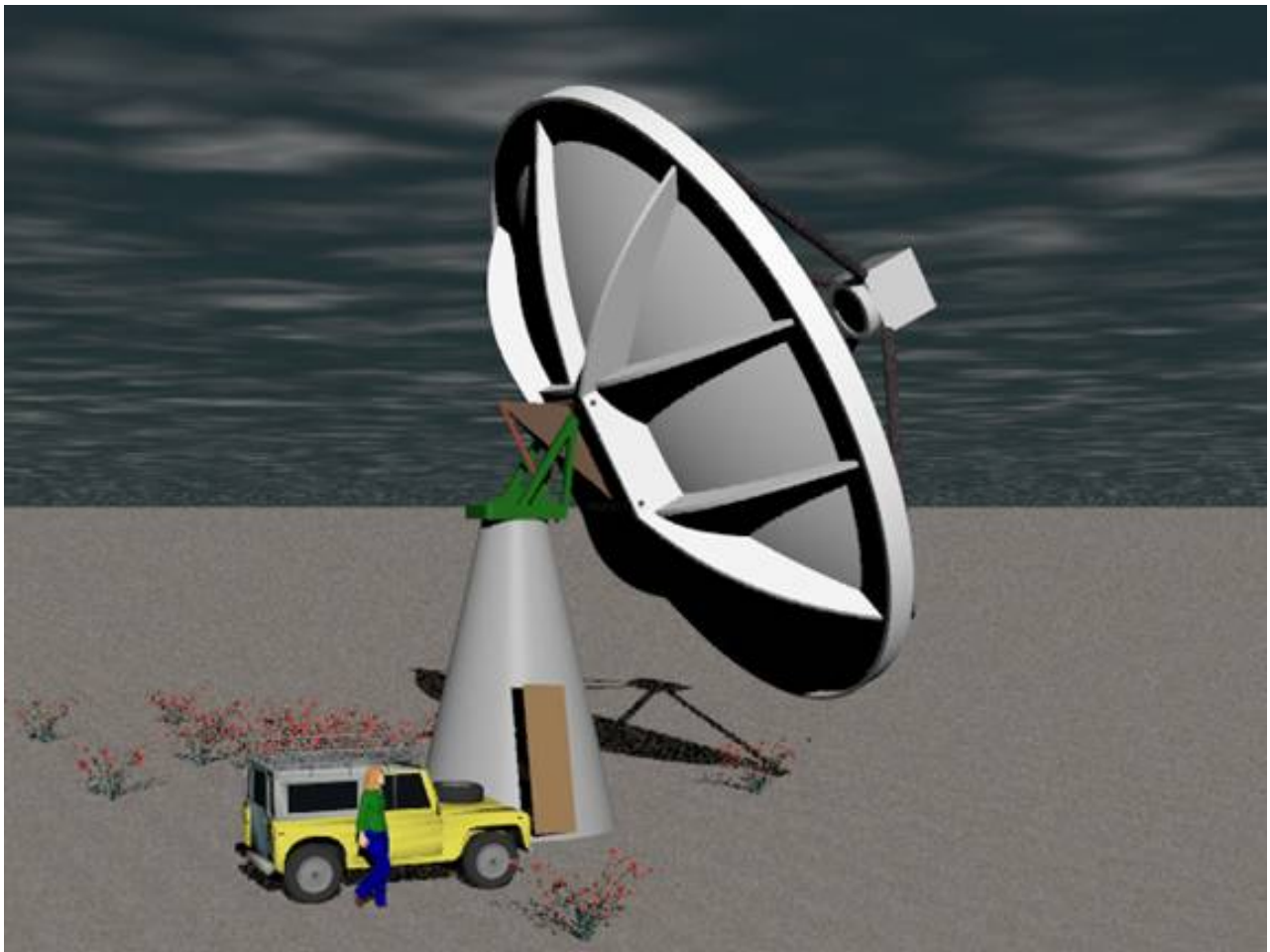
Figure 5. Rendering of a 12-m CART antenna currently under development at HIA DRAO.
